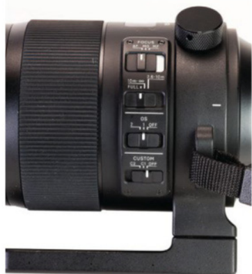
The three primary switches on the lens control (top to bottom): focus mode, focus limiting ranges, and optical stabilizer. The lowest switch selects a custom mode you program with the optional USB Block.
